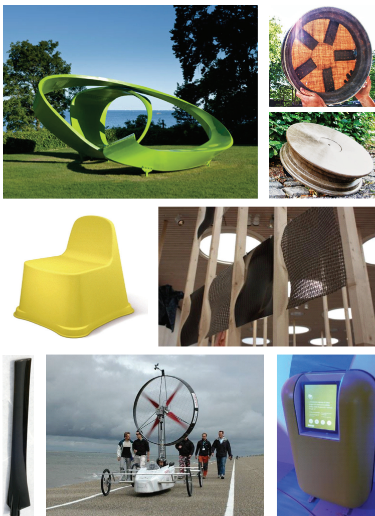
FIGURE 9: Examples of new applications of cellulose fiber composites: (top, left) sculpture, (top, right) wheel rim, (middle, left) chair for children, (middle, right) double-curvature panels, (bottom, left) small-scale rotor blade, and (bottom, right) exhibition stand. See text for more details.
